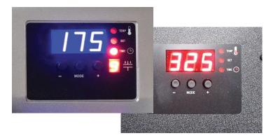
Press settings: Top Platen Heat: as low as possible (175°) Bottom Platen Heat: 325°- 350° Pressure: 9
