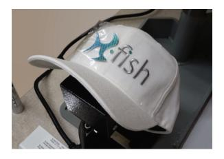
Lay the silicone pad on top of the emblem so that the emblem is centered under the pad and is completely covered.
