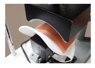
Remove the hat from the heat press and allow it to cool for 15-20 seconds. Slowly peel back the protective film from the emblem at a sharp angle.
