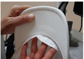
Place the hat on the bottom heat platen so that the sweatband is just below the edge of the platen.
